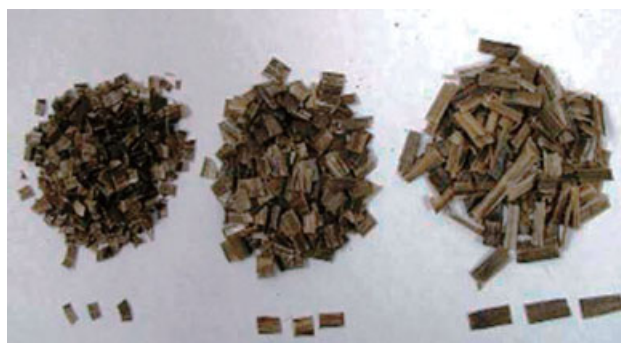
Figure 3 PPS/GF impregnated pellets with different length. [Color figure can be viewed in the online issue, which is available at www.interscience.wiley.com .]
